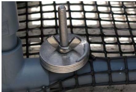
Figure 6: Trim Post with Stainless Steel Washer Weights
