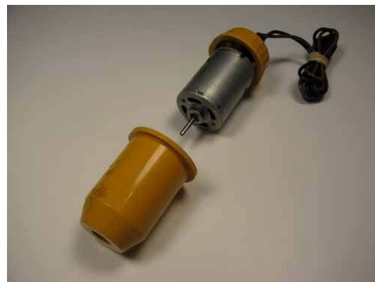
Figure 4: Cutting Too Close to the Motor Breaks the Waterproof Seal
