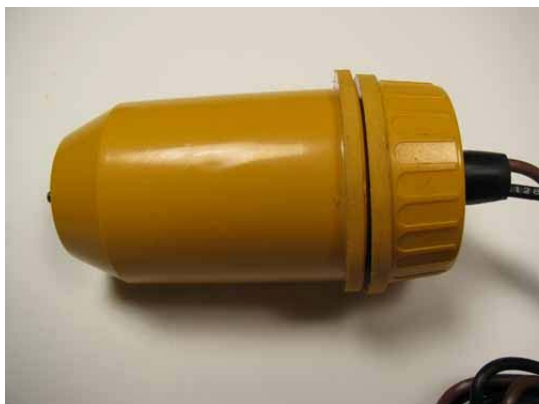
Figure 4: Cutting Too Close to the Motor Breaks the Waterproof Seal
