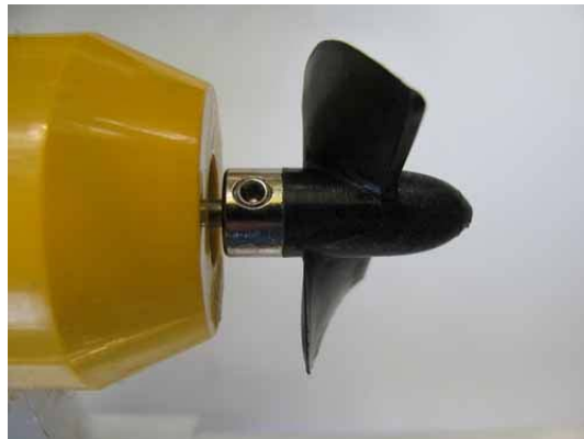
Figure 7: Traxxis #1583 Propeller Attached to the Bilge Pump
