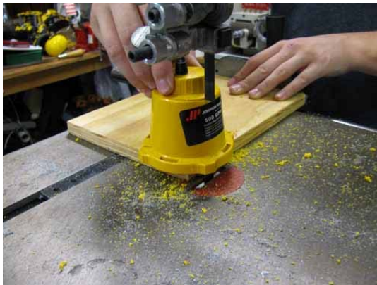
Figure 3: Cutting Off the Housing from the Motor
