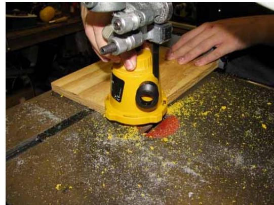
Figure 3: Cutting Off the Housing from the Motor
