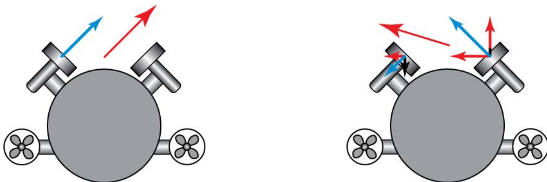
Figure 14: A Couple of Possible Movements if Thrusters Speeds Are Independently Controlled
