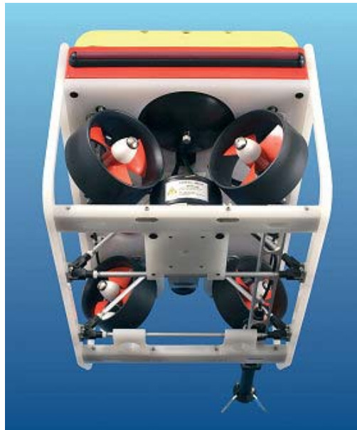
Figure 15: Four Vectored Thrusters for Horizontal Movement
