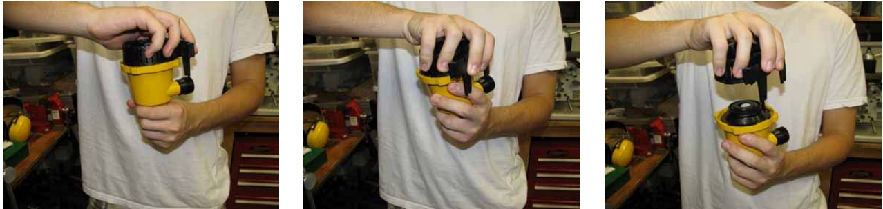
Figure 1: Twist Bilge Pump Unit to Remove
