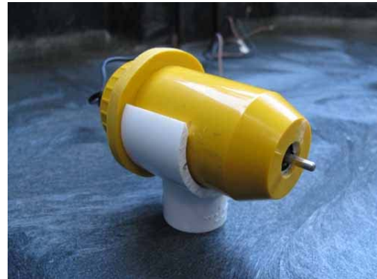
Figure 6: 1" PVC Tee and the Bilge Pump Seated in the Fitting
