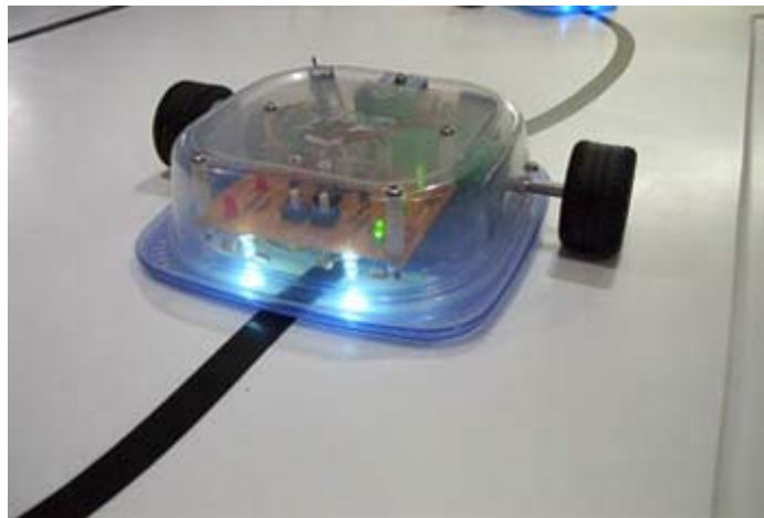
Sandwich – A Line Following Robot
